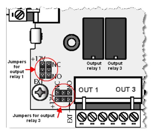
Each relay is associated with two jumpers. As shown below, a relay's left jumper configures the relay's load source (12VDC or External), and the right relay jumper configures the relay contact type (Normally Closed or Normally Open).
